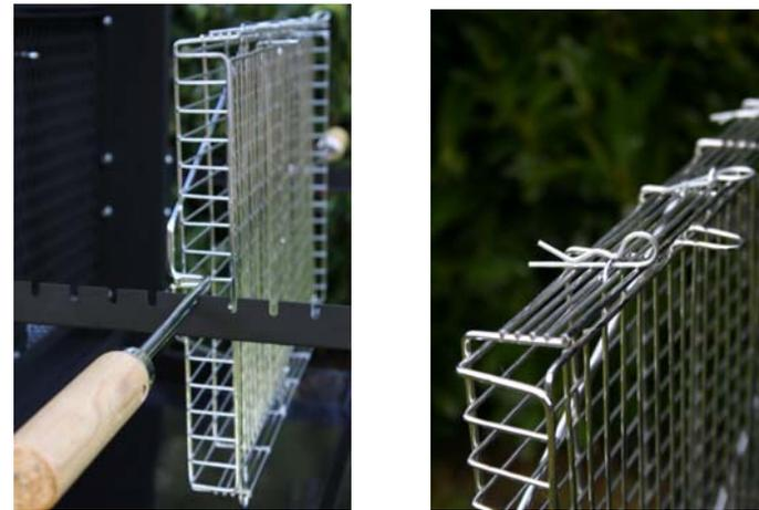
The food is held tightly in the cage grill by clamping it between the bottom grid and the lid of the cage grill (refer to the cage grill drawing). The height of each lid (2 lids per cage grill) can be adjusted on 4 positions so as to allow the cooking of food having various thicknesses (from 10 to 30 mm).
